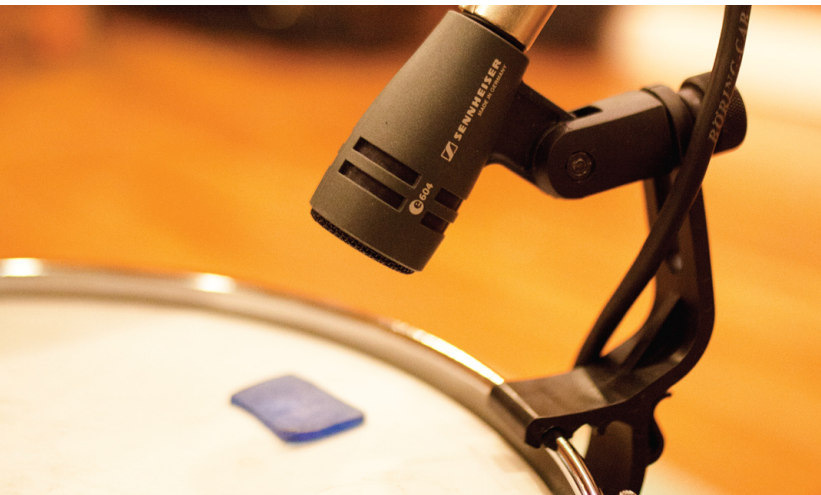
To augment the overhead and room mics, industry-standard close mics were employed, in conventional positions. Tommaso Colliva was surprised at how little the room influenced the sound captured by these close mics.
